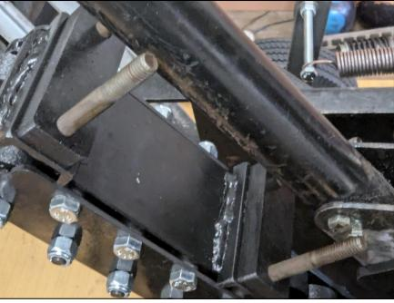
3) Slip the Ball Accelerator between the belt and the tube of the ball lift above the support bracket you just mounted. The long wheeled section goes downward toward the bottom pulley. Slide the Ball Accelerator down to the mounting tabs while flexing the ball lift belt down to line the bolts up with the Ball Accelerator tabs. Clamp it down with the provided mounting tabs and nuts. The units wheels will be around an inch from the bottom of the belt.
