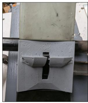
5) Slide the holding pad all the way down the wire tie into place on the lift arm. Push the wire tie through the upper slit of the holding pad and through the hole of the lift arm. Secure the wire tie on the back side and pull it tight.
