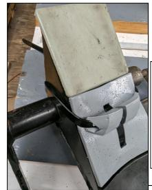
3) Rap the wire tie over the top of the lift arm tube as shown and zip it tight.
